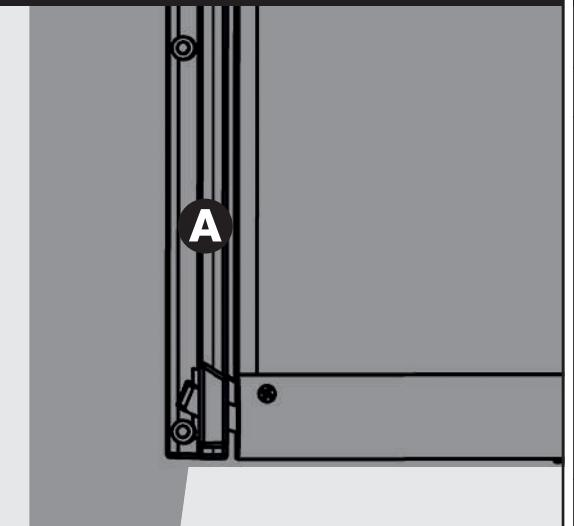
Insert door into position ensuring 'wing' is extended & secure within 'A' runner.
