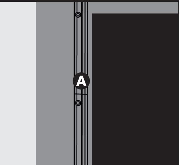
Align 'A' runner to left side of the opening on the chicken coop & secure by using large' screws. (use spirit level)
