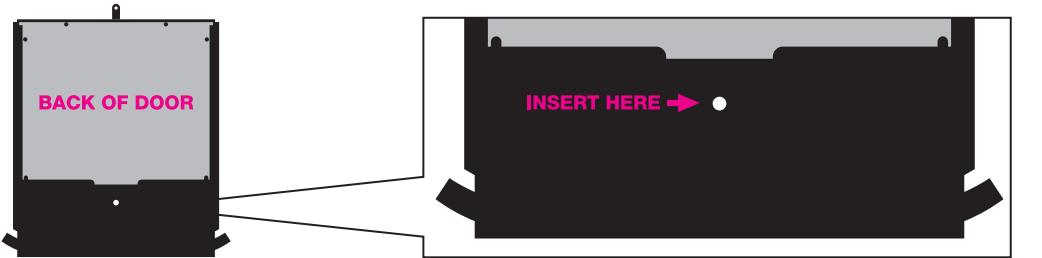
If worried about the locking mechanism freezing shut in extreme cold weather, this can be dis-engaged - simply ensure the door is in the fully up position, then insert a pin/screw/matchstick (not included) into back of unit to disengage locking mechanism. Door will now run freely without wings locking. Please remember to remove pin in order to re-activate when appropriate. Runners can also be lubricated in order to run freely in extreme weather.
