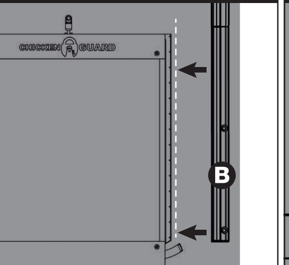
Align 'B' runner to right side of the door, leave a small gap to ensure door moves up & down freely. Secure by using 'large' screws. (use spirit level)
