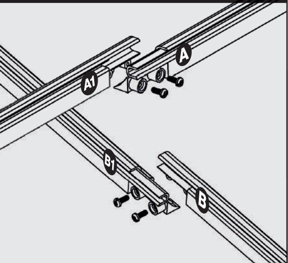
Align both 'A' runners & secure with 2 'small' screws. (repeat procedure for 'B' runners)
